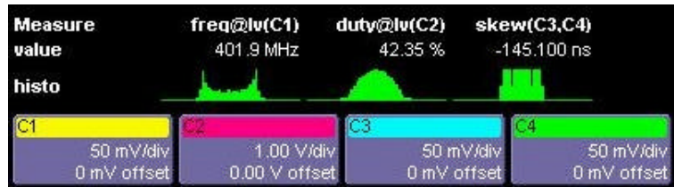
Figure 1 Histicons (histogram icons) showing frequency modulation, noisy duty cycle and a flat distribution of timing skew.
